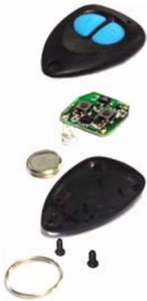
The batteries in the remote control will need to be replaced every 1 to 3 years, depending on usage. You are able to recognise when the batteries are low from when the range on the remote control reduces. Below describes how to replace the batteries in the remote control.
