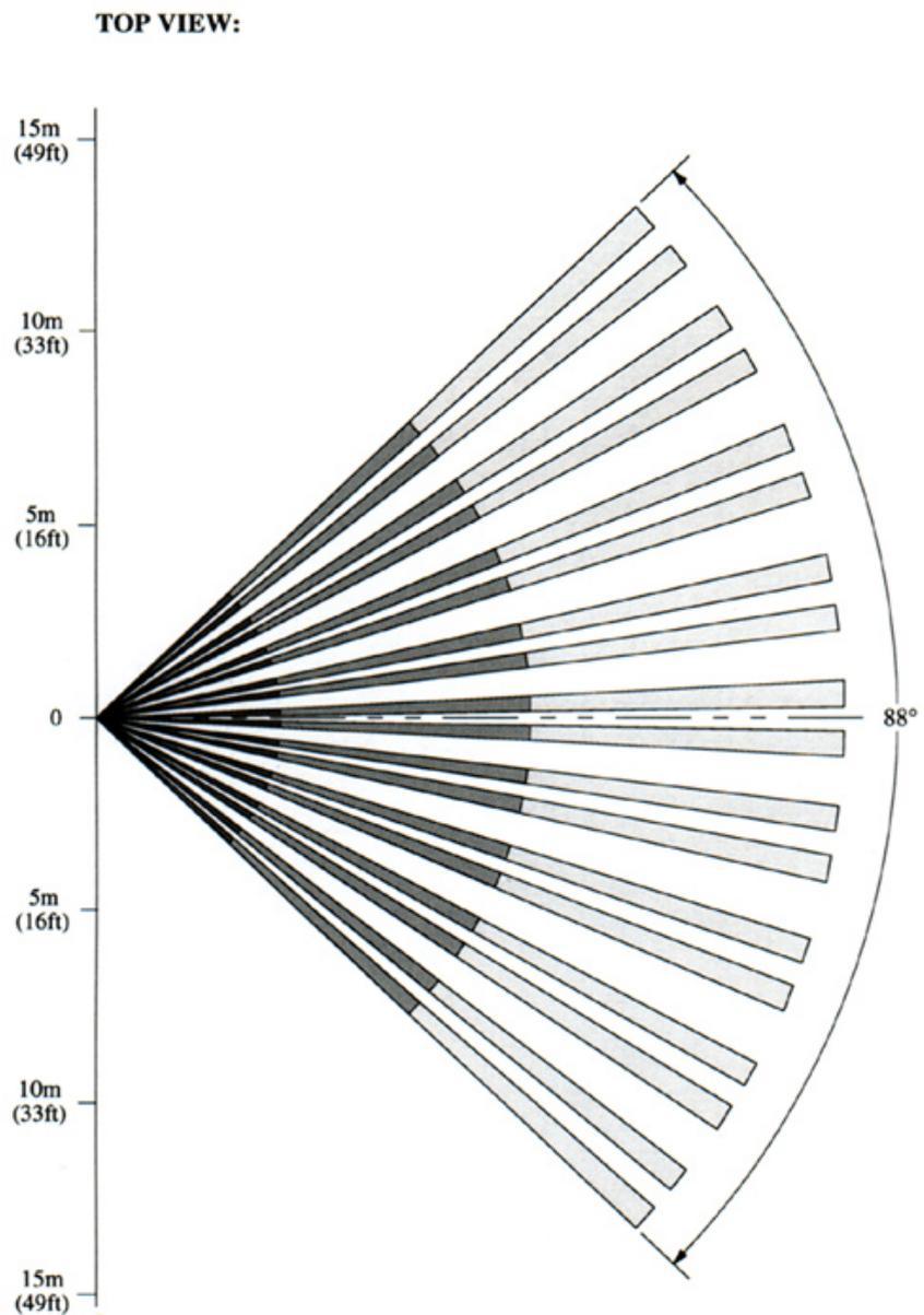
*Figure 10 – detection pattern in the optimal temperature environment*
