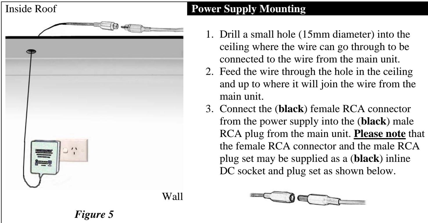
For a truly secure and professional looking installation have a power point installed in the ceiling by a qualified electrician so that the power supply (plug pack) is hidden and unable to be accessed easily. Another location for the power supply would be on an available power point at the rear of the fridge in the kitchen.
