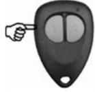
**Press 1 time** Within 3 seconds, press **Button 1** to select **detector programming**. You will hear **1 beep** as confirmation.
