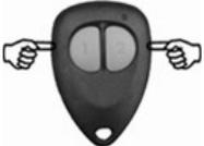
**Press both buttons for 3 seconds** Enter Programming mode by pressing **buttons 1 & 2** together for **3 seconds**. The siren will **beep 3 times** to confirm you have entered programming mode.
