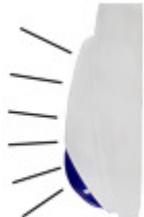
Wave your hand back and forth in front of the detector until the red light turns on. The siren will start screaming.
