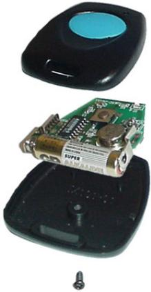
The batteries in the remote control will need to be replaced every 1 to 3 years, depending on usage. You are able to recognise when the batteries are low from when the range on the remote control reduces. Below describes how to replace the batteries in the remote control.
