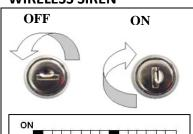
Set the Main Control Unit into wireless siren auto test mode by setting DIP switches 1 and 5 to ON.
