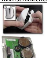
Power the detector opening the case and removing the plastic insert between the batterv terminals. Wait 3 minutes for the detector to warm up. During this time you can work out where you would like to locate your detectors.
