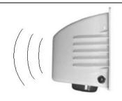
When this mode is entered the strobe on the siren will flash every 5 seconds, and the main unit will beep out the signal strength every 5 seconds. Note that the siren must be moved until a minimum of 3 beeps is heard from the main unit. Reset dipswitches to off.
