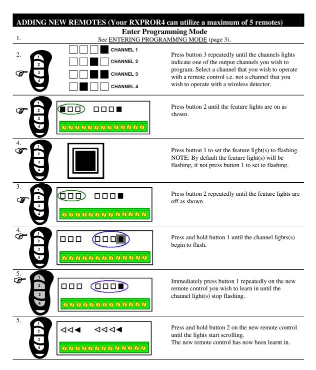
**Erasing Lost Remote Controls:** If you lose a remote control or perhaps have your car keys stolen, you can simply erase the lost/stolen remotes by repeating the procedure above 6 times. This will fill the system memory with remotes that only you have in your possession.
