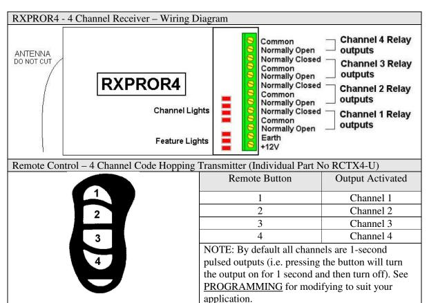
Antenna Mounting: For maximum operational range the antenna must be made vertical and straight.
