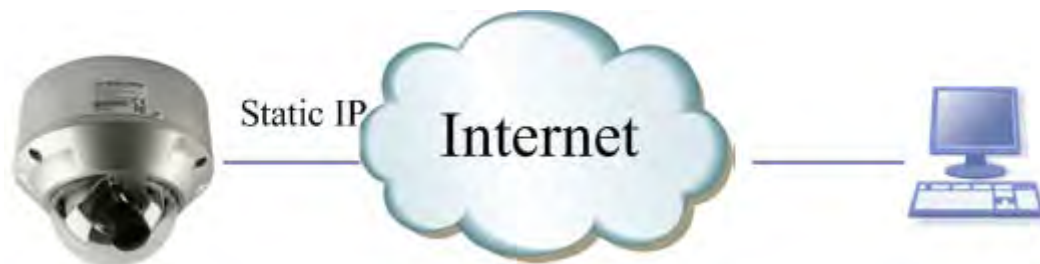
Fig.3.5.2 Static IP access IPC directly
