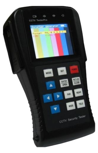
The VSCAMTESTERv2 is a Portable 2.8" LCD Test Monitor used to test, adjust and focus surveillance cameras whilst mounted in position. The unit will automatically select the appropriate signal mode (PAL or NTSC) based on the cameras output.
