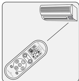
2. Press the "SET" button repeatedly until the air conditioner receives a signal from the controller. Normally indicated by a beep sound. Then press the "OK" button to confirm and set the correct code. Your RS10 remote is now ready for use.
