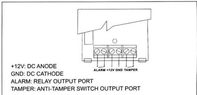
The dual passive infrared detector accords with national standards of P. R of China: GB10408.1-2000. It works by detecting human body's infrared spectrum. while receives body heat source signal from its movements in detecting area, the sensor sends out enlarged signal to MCU and MCU will sample continually, then output the signal after calculating to control the alarm port. This product is widely used in banks, warehouses, and houses etc.
