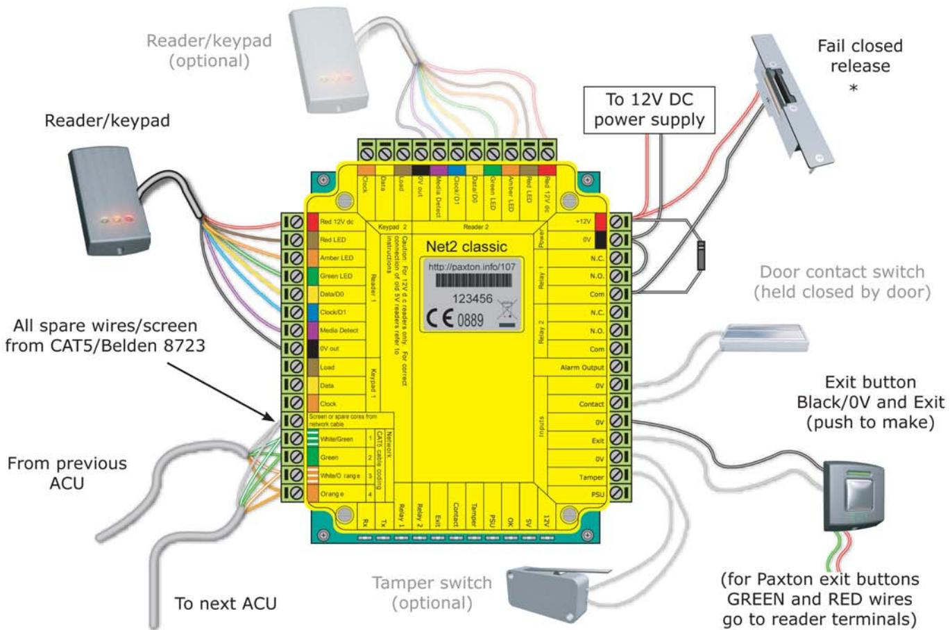
\* For a fail open lock (Maglock), the 0V loop wire is connected to the "N.C." terminal. (not the "N.O.")
