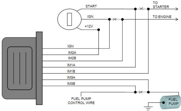
How to set up the on-board turbo timer:
