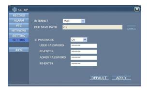
**INTERNET:** setting the code stream; the higher the code stream is, the clearer the remote image will be, but the network bandwidth must be high, otherwise the image may have a delay.
