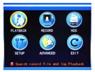
**Note:** The setup of all the submenus below will not be effective until "Enter" is pressed. The setup of this menu will be invalid if you exit directly. A significant characteristic of this product is when you move the cursor to any option, the prompting message of this option will be displayed automatically in the lower part of the screen.
