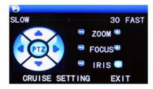
PTZ speed (fast or slow) can be controlled in this interface, zoom, focus and aperture is also controllable.
