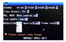
Channel: used to select if the video recording function is enabled for the corresponding recording channel.
