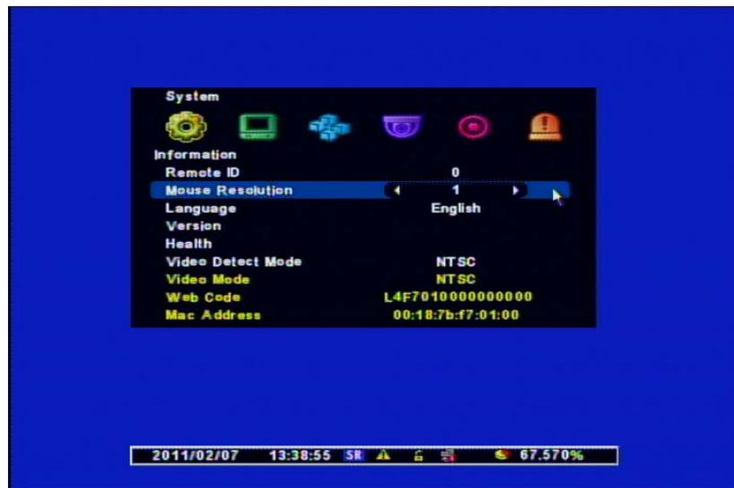
[1] **Remote ID** : Assign the ID of Remote Control so that user can separately control MunWlti DVRs with 1 Controller. (ID Range : 0 ~ 99)
