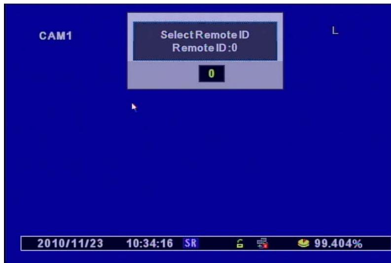
3) Press the "ID" Button on the Remote Control and then you can see the menu to change the DVR ID. (Refer to the above picture.)
