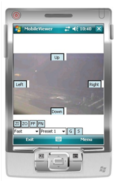
Figure 4.86. PTZF control screen
