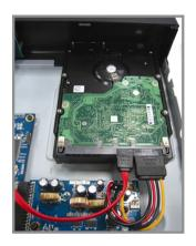
Step4: Align the screw hole on the each bracket with the screw hole on the each side of the hard disk as shown below, and fix the hard disk to the bracket with a hard disk screw supplied.
