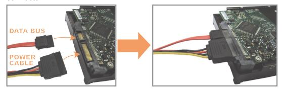
Step3: Make sure the PCB side is facing up, and place the hard disk between the hard disk bracket on the DVR base as shown below.
