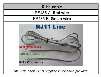
STEP 1: Get a RJ11 cable with the proper length to your connection.
