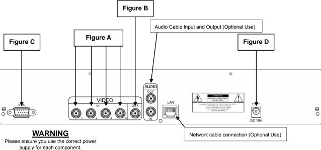
**DO NOT** plug the **19V DVR** Power supply into the cameras as this will damage them.
