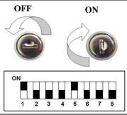
Set the Main Control Unit into wireless siren auto test mode by setting DIP switches 1 and 5 to ON.
