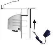
Screw the top 2 siren screws half way in and place the unit onto the wall supporting itself from the top 2 screws, then screw in and tighten the bottom two mounting screws then finish tightening the top two screws. Run the power supply wire through the roof to the closest power point, connect power supply and switch on.
