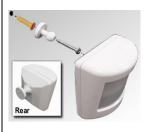
Now you can mount your detectors. Drill a 5mm diameter hole into the wall. Push the wall plug into the hole then screw in the mounting bracket. The detector can now be pressed onto the swivel bracket. Re-test the detector by opening & closing the case and then walking back forward in front of the detector. The main unit will beep each time the Red PIR Detection LED illuminates.
