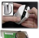
Power the detector by opening the case and removing the plastic insert between the battery terminals. Wait 3 minutes for the detector to warm up. During this time you can work out where you would like to locate your detectors.
