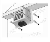
Drill mounting holes, (7mm diameter, 25mm minimum in depth) into the chosen wall. (If brick, use the green star plugs & press one into each hole. Now make a 12 mm diameter hole and push the wires through the wall and up into the ceiling for
