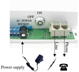
Remove cover plate then connect the phone line into the left side phone socket. If you are using a phone / fax / PC already at your available phone point, you may plug the lead from your existing device into the right side socket. Plug the power supply into a power point and switch on. Straighten the wire antenna for maximum wireless range. Now turn the main key switch to the ON position (do not press the remotes).
