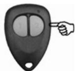
Press and hold **Button 2** (for approximately 3 seconds) on the **original** working remote control until the siren starts to beep continuously, then release the button.
