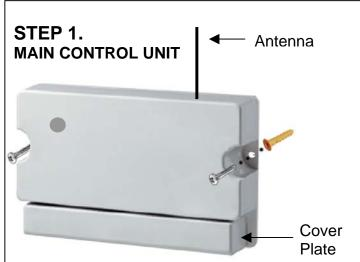
Choose a convenient mounting location to install the main control unit i.e. close to a phone outlet and power point. Drill mounting holes (7mm Diameter) into the chosen location. Mount the unit on the wall using the supplied screws and wall plugs.
