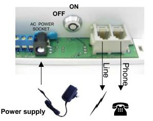
Remove cover plate then connect the phone line into the left side phone socket. If you are using a phone / fax / PC already at your available phone point, you may plug the lead from your existing device into the right side socket. Plug the power supply into a power point Straighten the wire antenna for and switch on. maximum wireless range. Now turn the main key switch to the ON position (do not press the remote).
