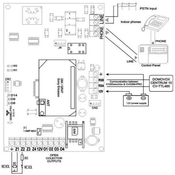
NOTE: The GSMBU-PRO can be power supplied from 12V
