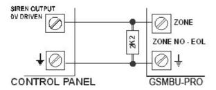
In order to trigger the alarm of the zone input when activating a 0V output, use the next wiring diagram. The zone must be programmed as NO-RFL.
