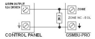
In order to trigger the alarm of the input zone when activating a 12V output use the next wiring diagram. The zone must be programmed as NC / EOL.
